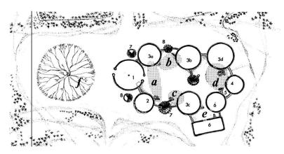
1) a circular, loadbearing wall pattern roofed with a conical system of rafters and thatch;
