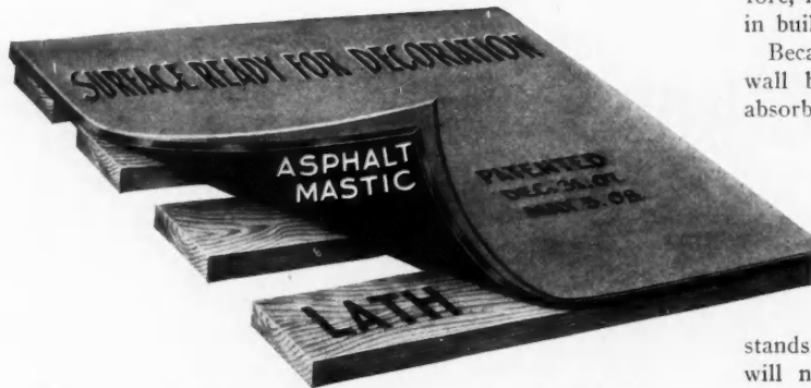
Illustration Shows the Construction of Bishopric Wall Board
