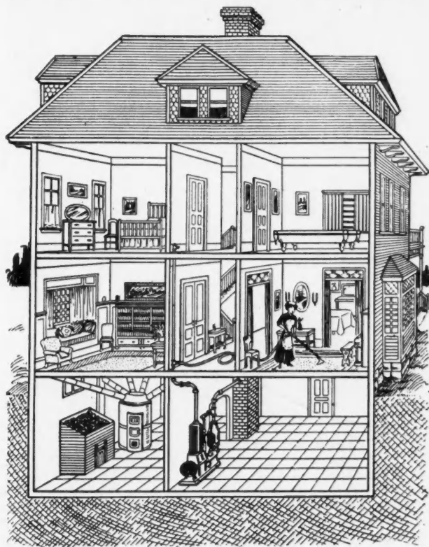
Sectional view of Residence, showing usual manner of installing a "Built-into-the-House" Vacuum Cleaning System.
