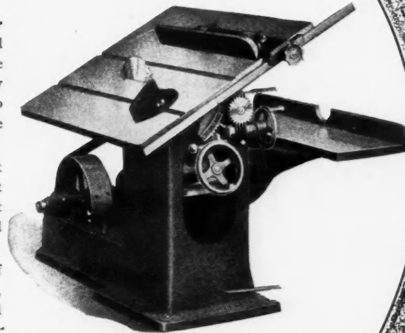
No. 2 Crescent Combination Saw-Table (Saw and Belt are included with this machine)
