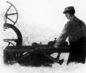
FAMOUS Universal Woodworker operated as Drum Sander.
