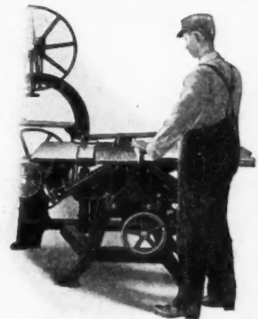
FAMOUS Universal Woodworker operated as Single End Tenoner.
