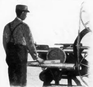
FAMOUS Universal Woodworker operated as a Disc Sander.
