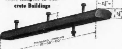
Trus-Con Pressed Steel Inserts are imbedded in the concrete during construction, saving expensive drilling after completion of the work. The long slots allow a wide variation in position. Special washers prevent bolts from turning in the slots. Write for details and prices.
