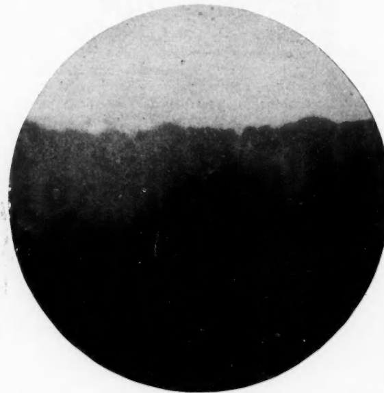
Cross Section of Lohmannized Sheet, Magnified 65 Times, Showing Permeation of Sheet by the Alloy
