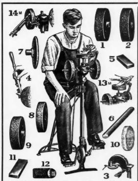
FOURTEEN MACHINES IN ONE. 1—Fine Dimo-Grit Wheel. 2—Coarse Dimo-Grit Wheel. 3—Universal tool rest. 4—Chisel and plane bit guide. 5—Dimo-Grit razor hone. 6—Dimo-Grit seythe stone. 7—Dimo-Grit saw gummer. 8—Felt polishing wheel. 9—Medium Dimo-Grit Wheel. 10—Cloth Buffing wheel. 11—Dimo-Grit oil stone. 12—Dimo-Grit pocket hone. 13M—Plane bit honing attachment. 14M—Twist drill sharpening attachment.
