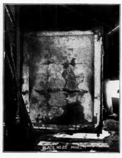
Photo of 5½" Partition—Cement Plaster on Metal Lath, 2×4 Pine Studs—After Two Hours Firing at 1912° Maximum Heat
