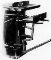
This attachment converts the borer into a hollow chisel mortiser, suitable for cutting mortises up to § inch square.
