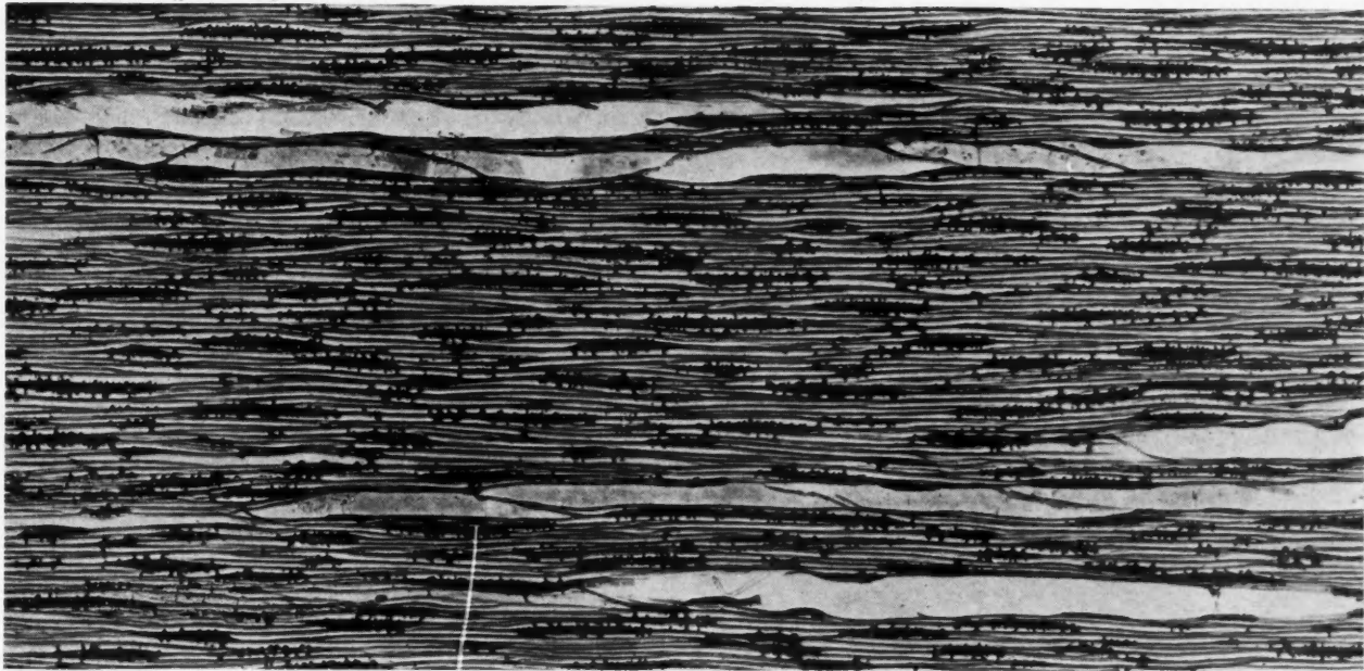
A Tangential Section of Yellow Birch Magnified Fifty Times. Made by the Forest Products Laboratory, Forest Service, U. S. Dept. of Agriculture, Madison, Wis.
