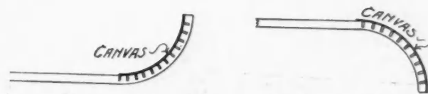
Wood Veneer or Canvas Glued on Holds Curved Shape
