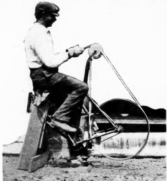
A Serviceable Grinder Made of An Old Bicycle
