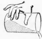
Water poured off, leaving white lead and linseed oil.
