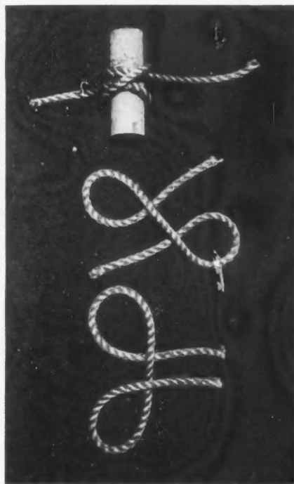
Fig. 3. How the two half-hitches are tied. Be sure to get this just right.
