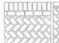
When double squares are laid "basket pattern," the necessary allowance for joints adds interest
