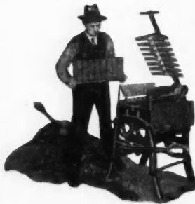
16 perfect clean cut brick in one operation. Time—one minute, 1/2
