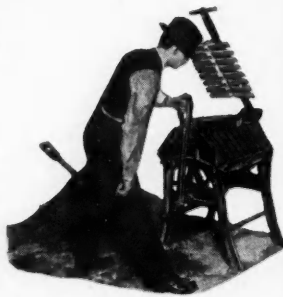
One Throw of the Lever Delivers Eight Brick on each side of the machine
