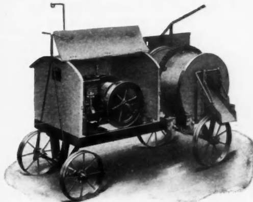
CAPACITY—5-ft. batch, easily fifty cubic yards per day.
