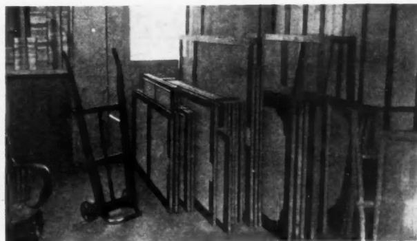
Shop store-room, showing order of screens all ready to ship out. This room contains all odds and ends, so that there is nothing in the way in the shop proper. Even the line shaft is under the floor, out of the way.
