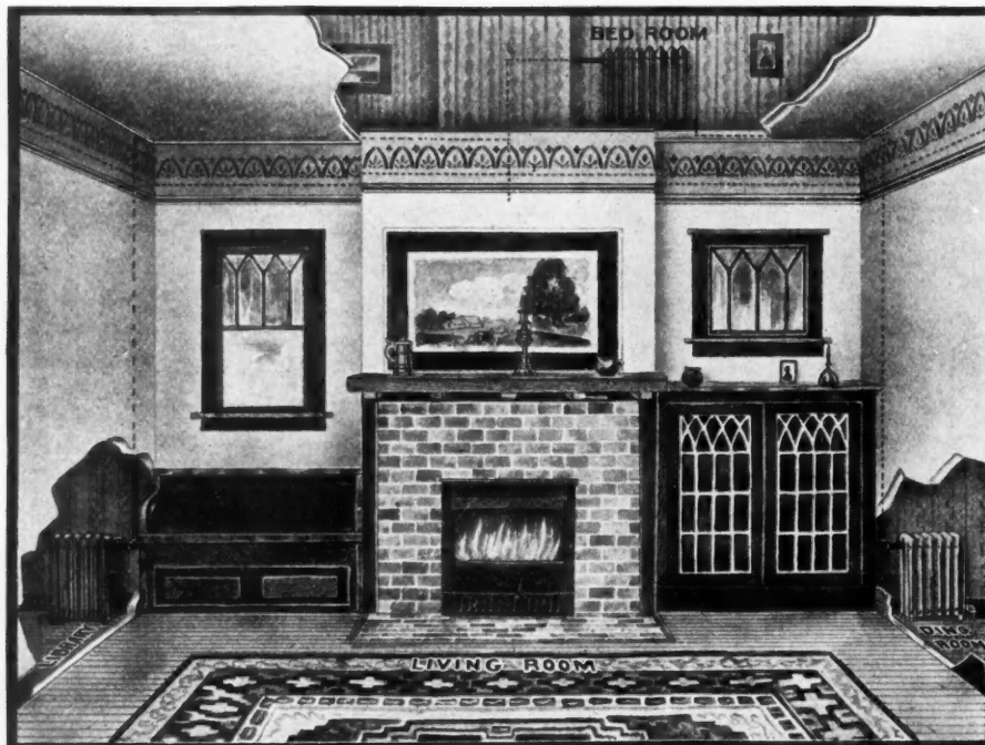
Section of Residence Showing the Heater in Fireplace in Living Room, with Hot Water Radiators in Library, Dining Room and Bed Room.
