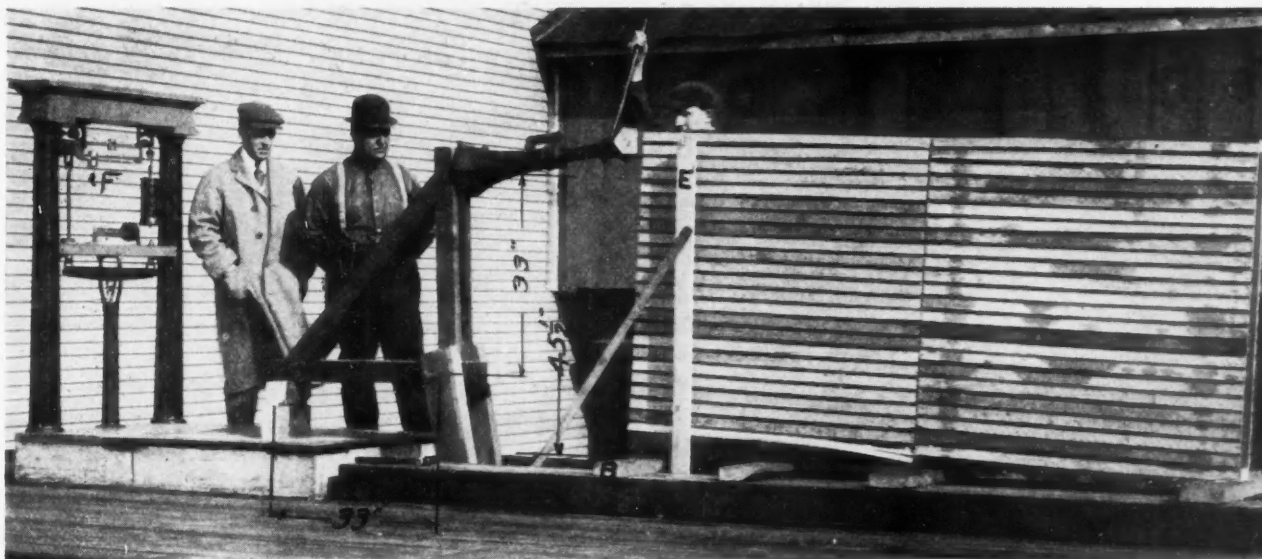
Fig. 3. Testing Frame with Stucco Board on Both Sides Withstanding Test Pressure of 2650 Pounds with Deformation of Only 1\frac{1}{16} In.
