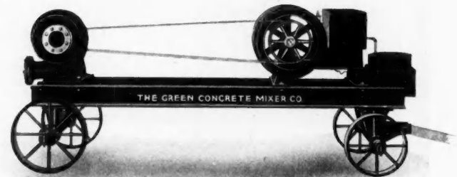
The Green Truck Equipped with Centrifugal Pump.
