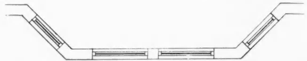
Plan of Bay Window Which is to Terminate in Dormer on Roof.
