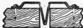
End view showing joint open. Provides for expansion or contraction of the siding so nails will not work loose.
