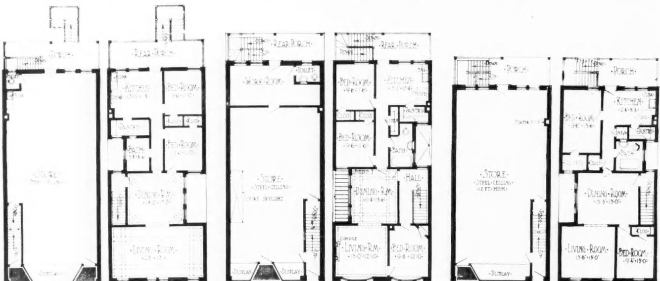
Floor Plans of Design No. 6788. Floor Plans of Design No. 6789. Floor Plans of Design No. 6790. General Floor Arrangements of Three Store Buildings Shown Above and Also Arrangement of Rooms in Apartment Above Each Store.
