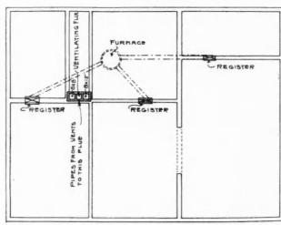
Suggestions for Placing Heat Ducts in Walls.
