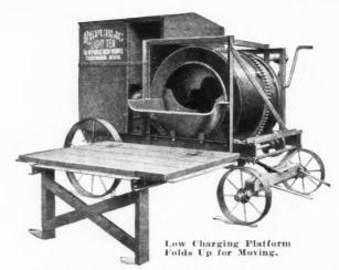
justing bearings to avoid binding of the working parts. The platform folds up for moving, making the mixer instantly available when placed on the job.
