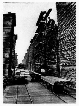
Gasoline Power Lumber Piler Used to Reduce the Cost of Piling and Unpiling Lumber. Capacity is Claimed to be 10,000 Feet of Lumber per Hour.
