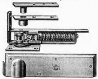
The most durable hinge of its type; holds the door open when swung to 90 degrees at either side. The spring-action can also be entirely released as long as desired so that the door will swing free, without spring-action, in either direction, by inserting a wire nail (when the door is open) into a hole provided in the side plates for that pur-The spring-action can be restored by withdrawing
