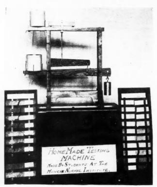
Machine for Testing Concrete Briquettes in Flexure, Made by Students at the Muncle (Ind.) Normal Institute.
