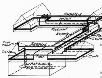
Fig. 6. Arrangement of Heat Coils
