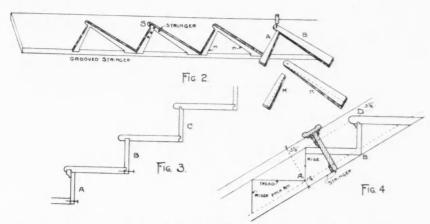
Fig. 2. Showing How to Groove a Stringer. Fig. 3. Different Methods of Connecting Risers and Treads. Fig. 4. Finding the Width of a Stringer.
