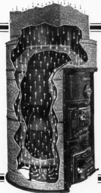
Sectional View, showing Double Casings and Circulation of Air
