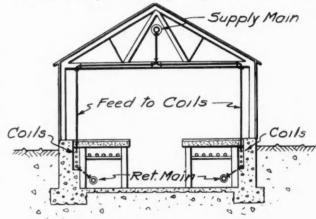
Fig. 2. Typical Section Thru Green House
