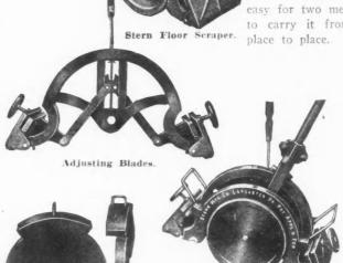
With the handle in an upright position it is possible for the scraper to be used in narrow rooms and halls where scraping is often found very difficult.
