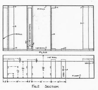
Construction of Combined Bed and Wardrobe as Shown in Section.
