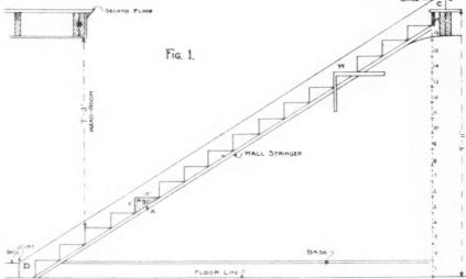
Fig. 1. Elevation of a Housed-Wall Stringer,
