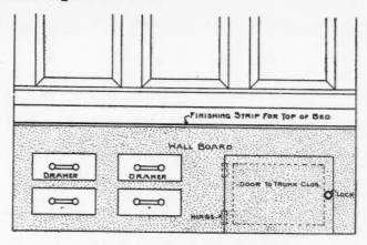
FIG. I. ELEVATION OF BED IN SLEEPING PORCH. Front Elevation of Combined Bed and Wardrobe.
