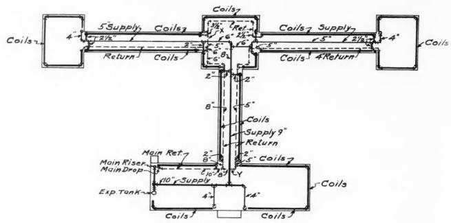
Fig. 7. Plan View of Heat Piping System.
