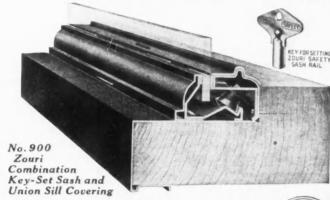
The Zouri Safety Key-Set Sash (with Union Covering) No. 900 is shown here to be free from dangers of direct screw pressure, or a resilient rabbet. Its inner member is rigid. The Union Sill Covering, extending from inner side of plate glass to lower edge of sill, has no joints, no perpendicular screws, no sill deterioration, because leakage is impossible. Made in solid copper.
