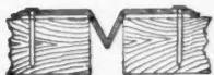
Shows end view of Batten with the joint open and siding contracted. Chief Battens automatically accommodate expansion and contraction.
