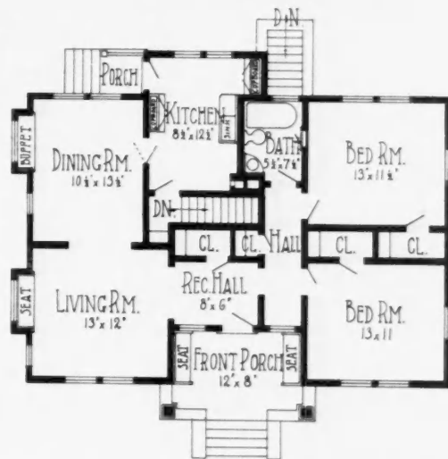
Floor Plan of Bungalow. Size 27 Feet by 40 Feet.
