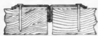
Shows end view of Chief Galvanized Batten with joint closed. Siding expanded. Note position of the batten in the crack.
