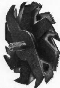
Showing position of cutters on mandril.
