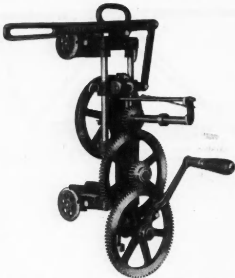
Lock Mortiser Which May be Operated at 1200 R.P.M.
