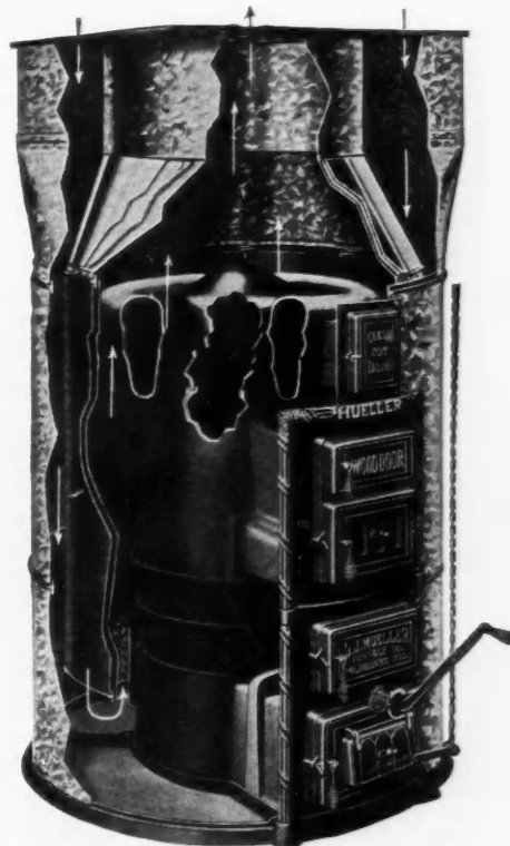
Sectional View of Mueller Pipeless Furnace
