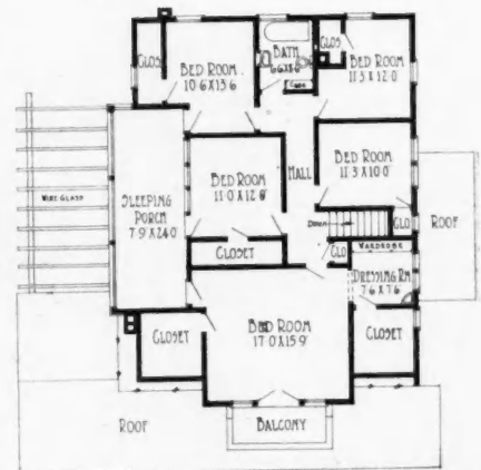
First and Second Floor Plans of House Shown in Perspective Below. Size, 34 by 43 Feet.
