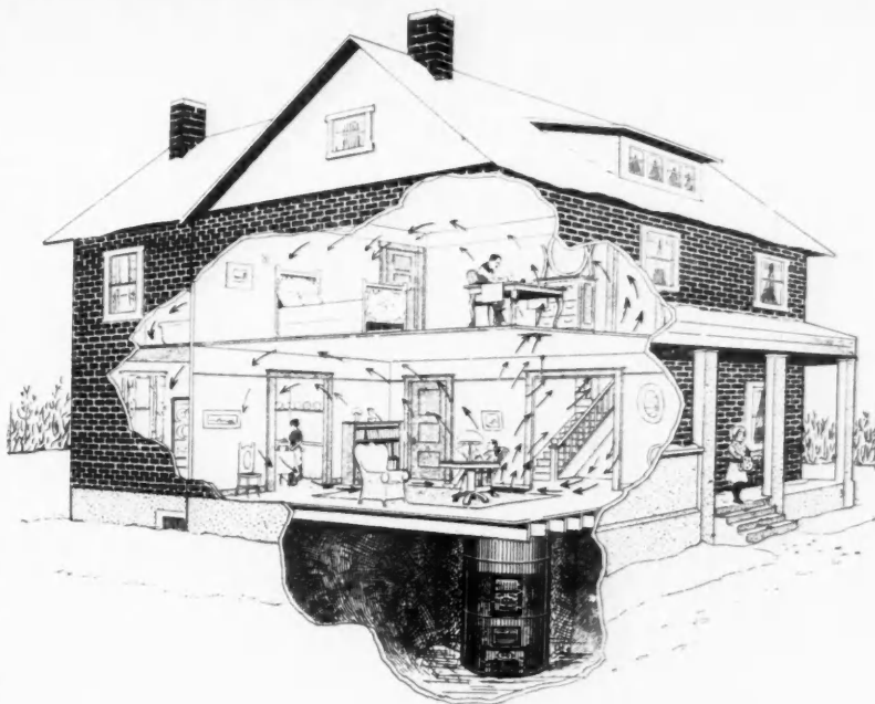
Two-Story Houses as Well as Cottages Are Successfully Heated with the Pipeless Furnace. The Saving in Fuel Is Important.
