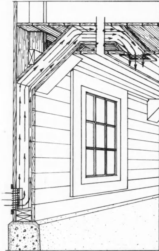
Perspective Sketch and Detail of Fresh Air Flue for stable with cows facing in. Fresh air is brought in just above the foundation, is carried up to the ceiling and across between joists to ceiling register at the center aisle.
