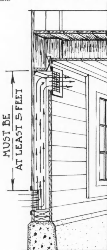
Detail of Fresh Air Flue in stable with cows arranged to face out. Fresh air should always be admitted in front of the cattle at the ceiling and foul air taken out back of them near the floor. The 5-foot height between the inlet and outlet for fresh air assures an upward current of air at all times and prevents a back draft.
