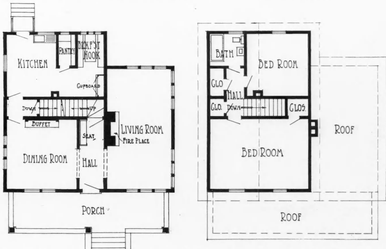
First and Second Floor Plans of House After Remodeling, Showing Large Modern Living Room Added to the First Floor, and Second Floor Rearranged to Provide a Bathroom.
