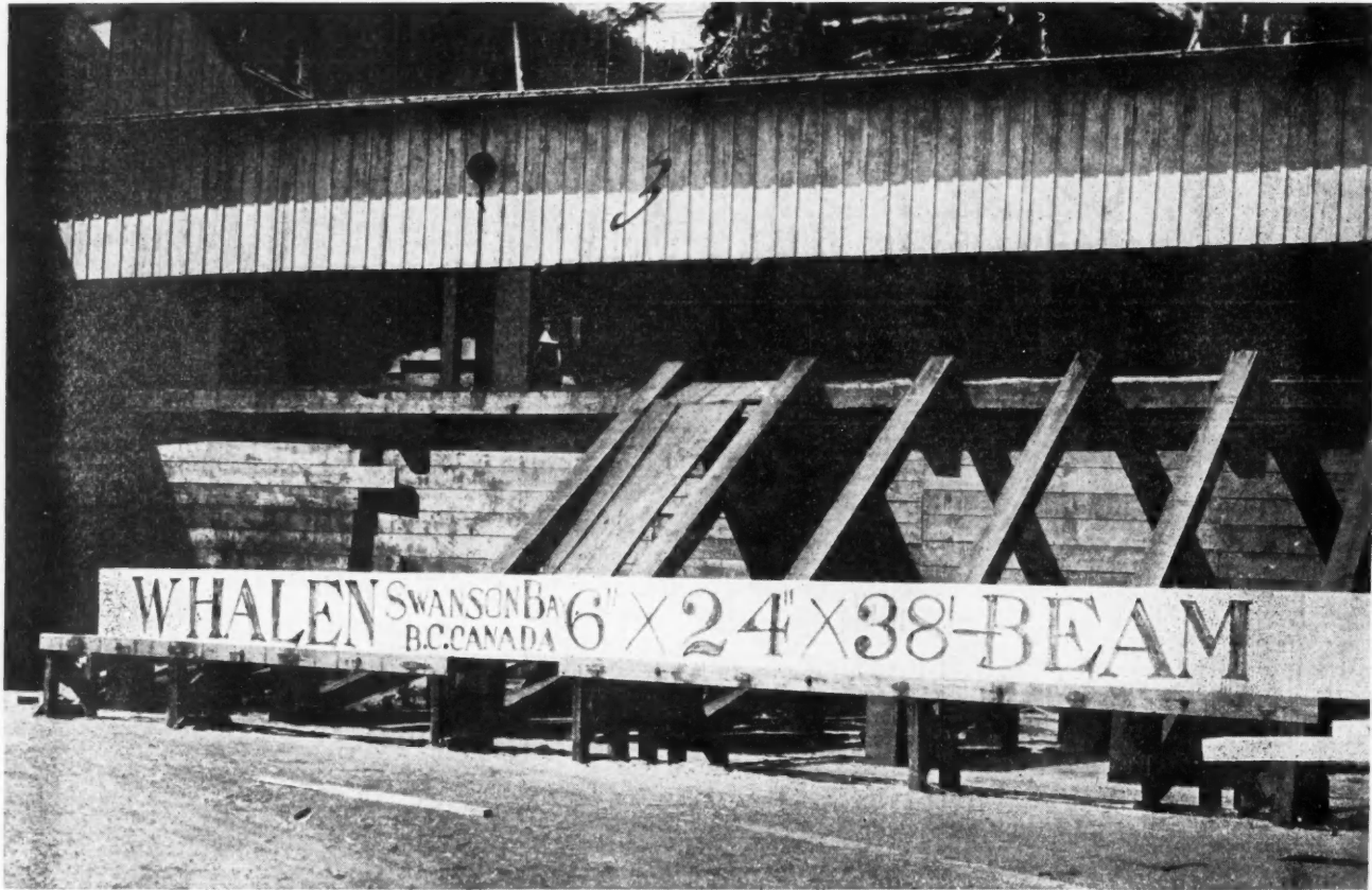
Here is a Perfect Piece of Airplane Spruce, 6 by 24 Inches, 38 Feet Long, Containing 456 Board Feet, Produced by the Whalen Pulp & Paper Co., Ltd., at Their Swanson Bay, B. C., Mill. Another Big Stick Produced at the Same Time Measures 6 by 22 Inches, 38 Feet Long, and the Statement is Made at the Mill That These Are the Two Largest and Most Perfect Sticks of Spruce Airplane Stock Yet Produced. The Whalen Pulp & Paper Co., Ltd., Have Mills at Howe Sound, Swanson Bay, and Quatsino Bay, All in British Columbia.
