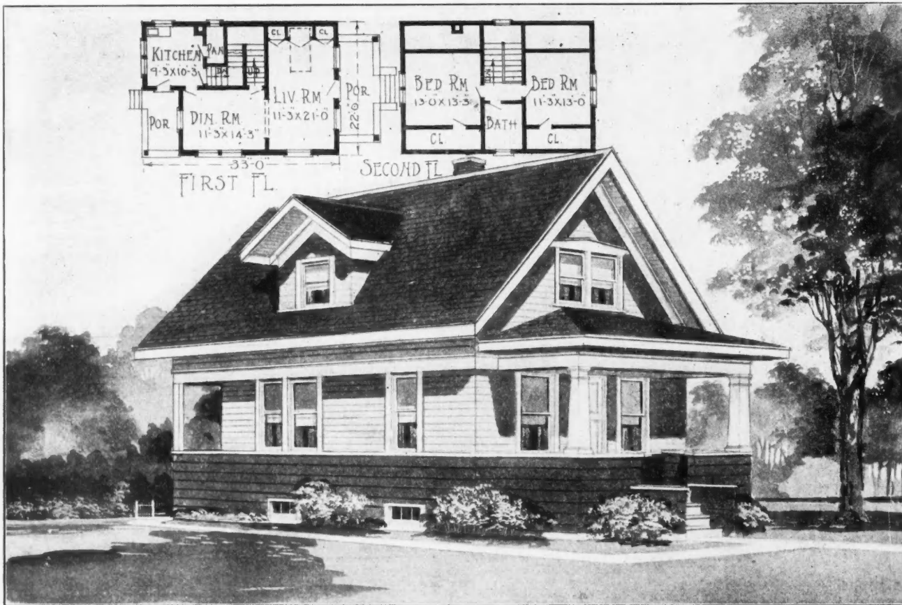
Architect's Perspective Sketch of Industrial Housing Cottage. Complete Working Plans for Which Are Presented in the Blueprint Pages Following. This Rendering Shows Wood Construction with Wide Boards and Beveled Siding. Three Alternate Exterior Designs Featuring Other Materials of Construction Are Shown on Sheet No. 1.
