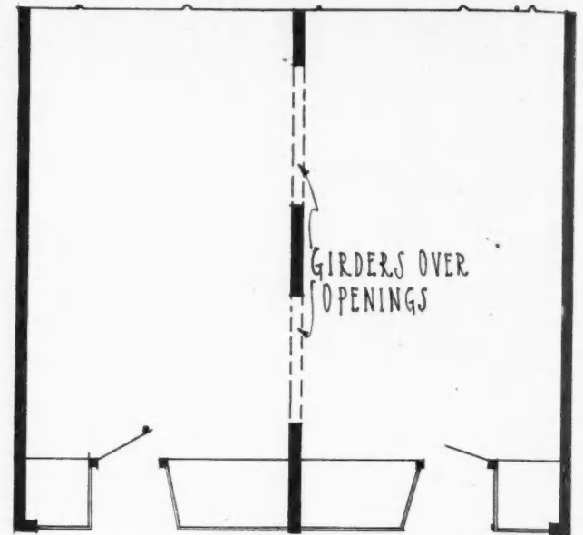
The Stores Joined by Piercing the Wall.
