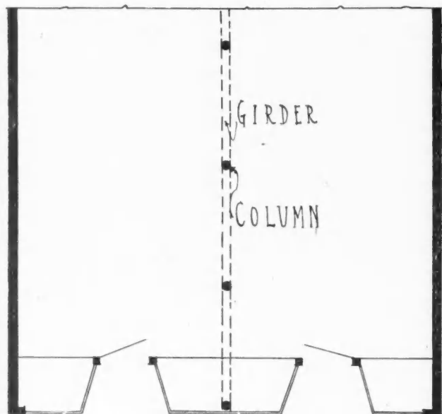
The Wall Entirely Removed and Columns and Girders Used to Carry the Upper Walls.
