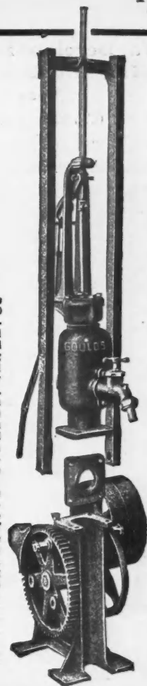
Goulds Fig. 1680 - Combined Deep Well Working Head and Jack Easy to install. Flange (in center) screws on end of well pipe which fits into recess in base that supports the pipe, allowing top part of pump to be installed with ease. For filling tanks not more than 190 feet above water level. For engine, windmill or hand operation.
