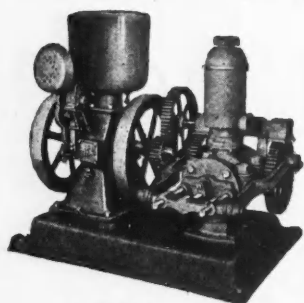
Force Pumping Outfit, 2½, 4½, 6, 8, 10 H. P. Capacity 800 to 7200 gallons per hour.
