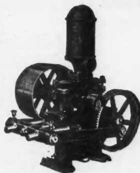
Goulds Pyramid Pump Fig. 1531 - For open or compression tank water systems. For direct or belted drive from electric motor or belted drive from gasoline engine. Capacity 6 to 114 gal. per minute against pressures up to 75 lbs. or elevation up to 175 ft.
