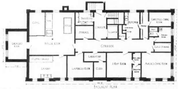
Every Facility for Hospital Operation Is Provided in the Basement.
