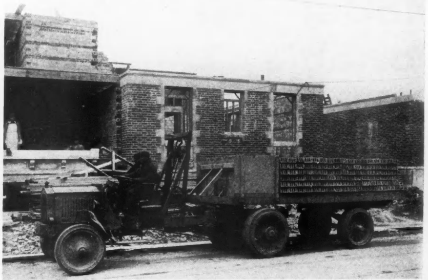
There Are Ten Tons of Bricks on This "Fruehauf" Trailer, Attached to a Five-Ton "Packard" Truck, Owned and Operated by the Delta Brick & Tile Co., Detroit, Mich.
