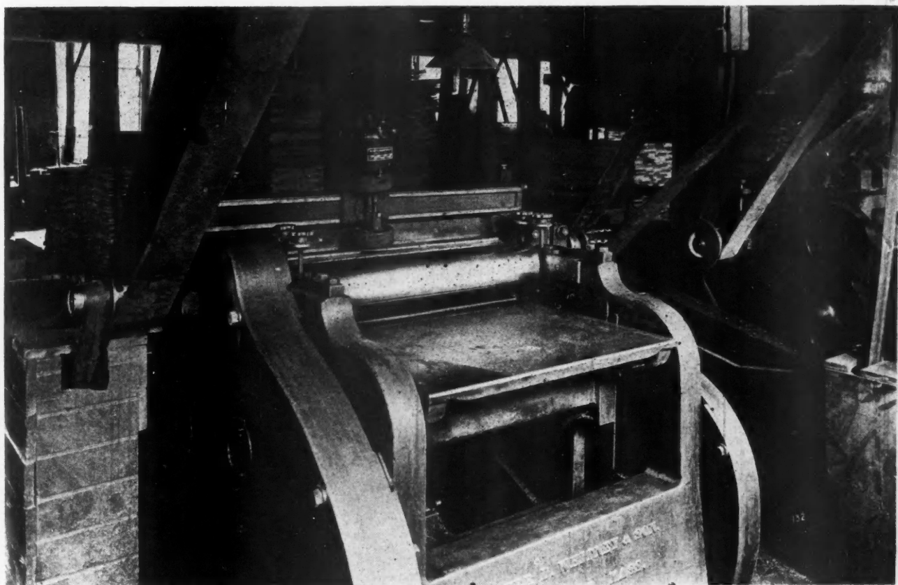
The Planer in the Foreground of This View of the Interior of a Woodworking Shop Is Equipped with a Little Sharpener Tool That Keeps the Knives in Fine Condition. They Are Sharpened in Place Which Saves Time It Would Require a Workman to Remove the Knives and Also Keeps the Planer in Operation Practically Continuously.
