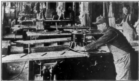
Routing a Stair Stringer. The Operator Is Guarded by the Skirt of the Machine, Which Makes It Impossible to Come in Contact with the Cutters.
