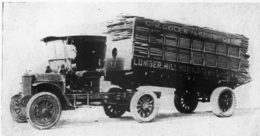
Two-Ton "Federal" Truck and Five-Ton Trailer Equipped with "Martin" Rocking Fifth Wheel, of C. B. Coles & Sons Co., Camden, N. J. This Combination Gives the Coles Concern a Piece of Hauling Equipment of Large Capacity at a Minimum of Cost.
