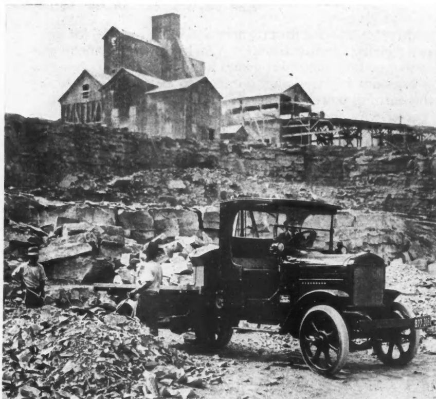
This Three-and-a-Half Ton Stewart Truck Is Hauling the Stone Direct from the Quarry to the Job for a Buffalo Contractor. It Has a Utility Body Which Can Be Fitted for Carrying Sand and Cement by Adding Sideboards.
