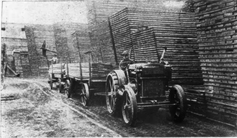
A New Stunt in the Lumber Yard. This "Case" Tractor Has Been Found Very Useful in Hauling Around Trailers to Be Loaded. When Ready They Are Brought to the Shipping Yard Where a Motor Truck Takes Them to their Destination.
