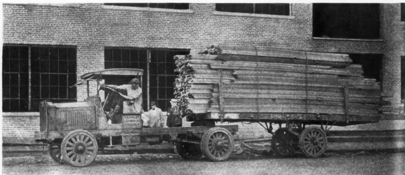
Carrying an Extra Heavy Load of Lumber on a Semi-Trailer Pulled by a Five-Ton "Standard" Truck. Lumber Dealers Find This Combination Very Efficient and Today More Than Ten Thousand Dealers Are Operating Trucks in the Lumber Business.
