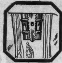
Fig. 2. Complete Wedge Inserted in Hammer Handle.
