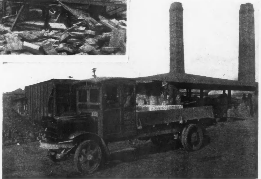
One of the Most Effective Assistants of the Building Supply Dealer and Contractor Is the Motor Truck Equipped with Special Dumping Body.
