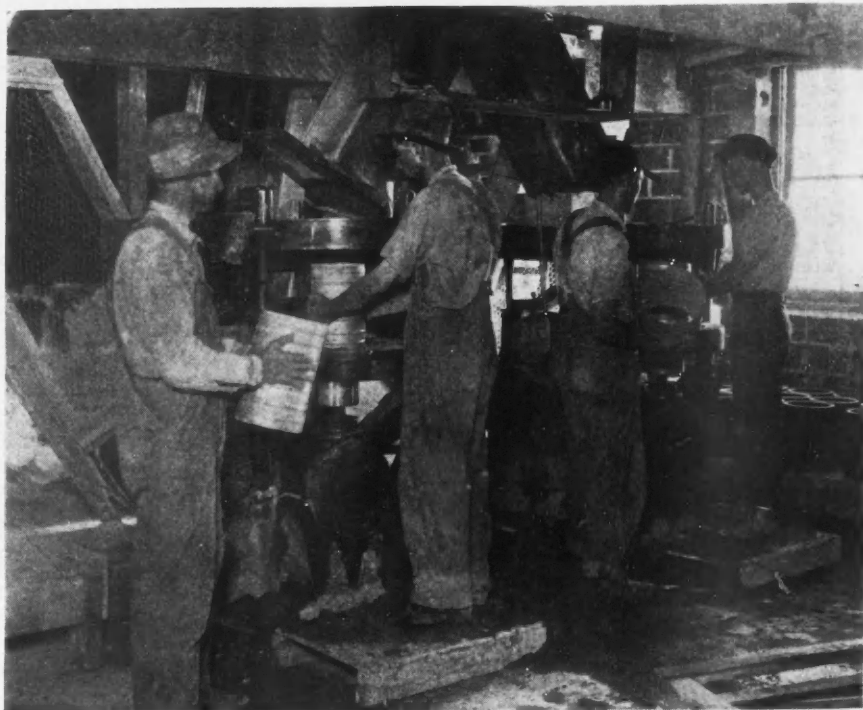
Making Concrete Drain Tile on Power Concrete Products Machinery. This Type of Machinery Has Been Perfected to the Point Where a Plant Can Turn Out Many Thousand Units Per Day.
