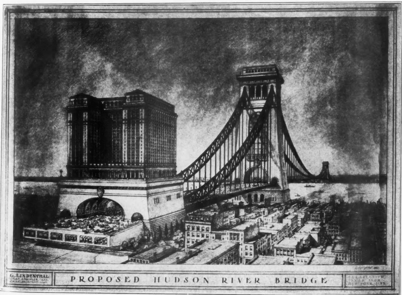
Drawing of Proposed Hudson River Bridge Which Will Be Largest of Its Kind in World. The Central Span Will Be 3,240 Feet Long. The Towers on Each End 840 Feet High. On the New York Side a Skyscraper Will Be Built. All Steelwork Will Be Coated with Bronze.
