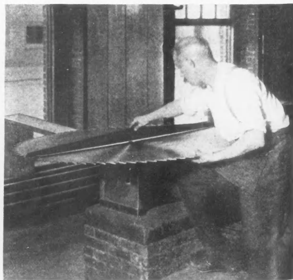
Fig. 2. Appearance of Saw That Has Lost Its Tension. This Needs Hammering with Round-faced Hammer Along Lines Shown in Fig. 3A.
