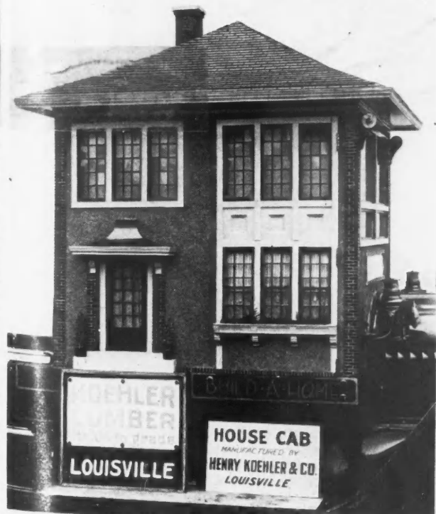
Close up of Driver's Cab Built to Resemble a Complete House in Miniature. The Driver Enters the Door on This Side Hung on Hinges. The House Is Covered with Stucco and the Roof with Miniature Blue Slate Asphalt Shingles.
