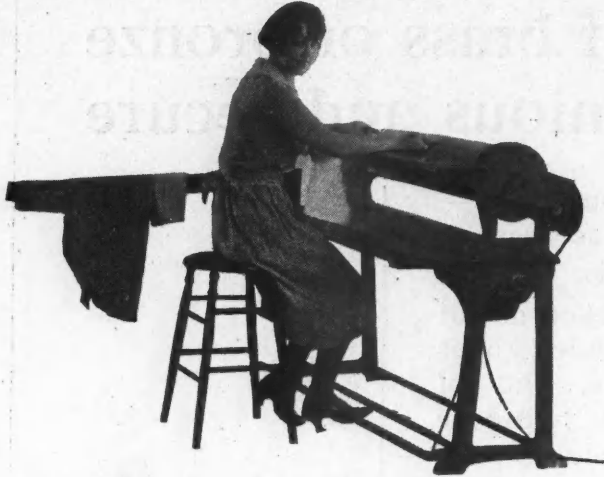
A Foot Control Which Runs Along the Entire Length of This Ironer Leaves Both of the Operator's Hands Free to Guide the Material Through the Ironer.
