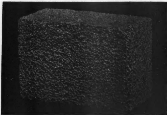
Millions of Tiny Air Cells Are Confined in This Insulation Formed of a Gypsum Product and Water.
