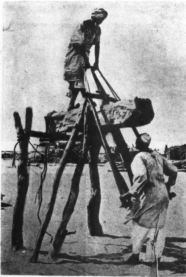
In the Sudan, Africa, This Crude and Primitive Method of Sawing Is Still in Common Use.
