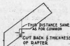
Fig. 38. Lengthening Seat Cut for Rafter. Fig. 39. Beveling Hip and Valley Rafters.
