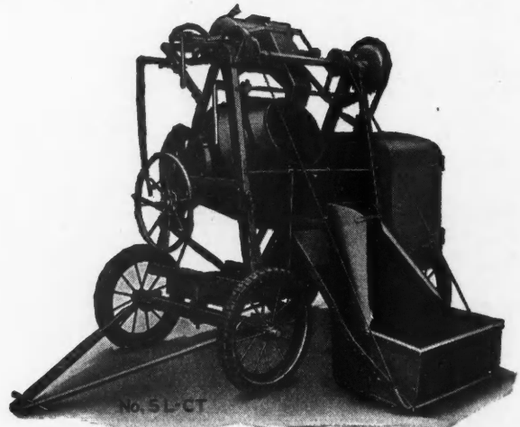
One of a Series of Mixers Which Has Been Added to a Well-Known Line of Concrete Machinery to Supply the Demand for an All-Around Mixer.
