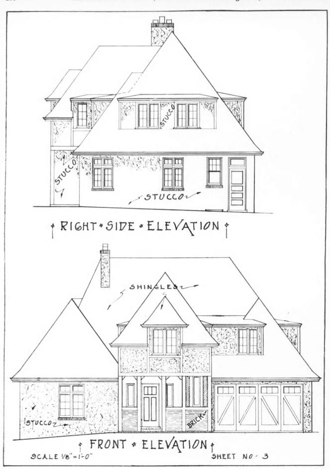
The Front and Right Side Elevations of Our Front Cover Home, Showing the Window Treatment Which Is Carried Out in the Garage as Well as in the Other First Floor Rooms.
