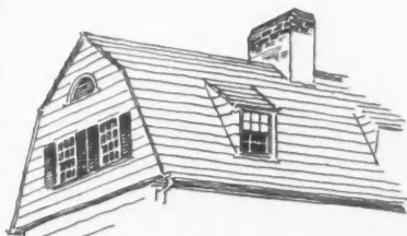
FIG. 7. THE GAMBREL & DORMERS AS A SHINGLED UNIT.
