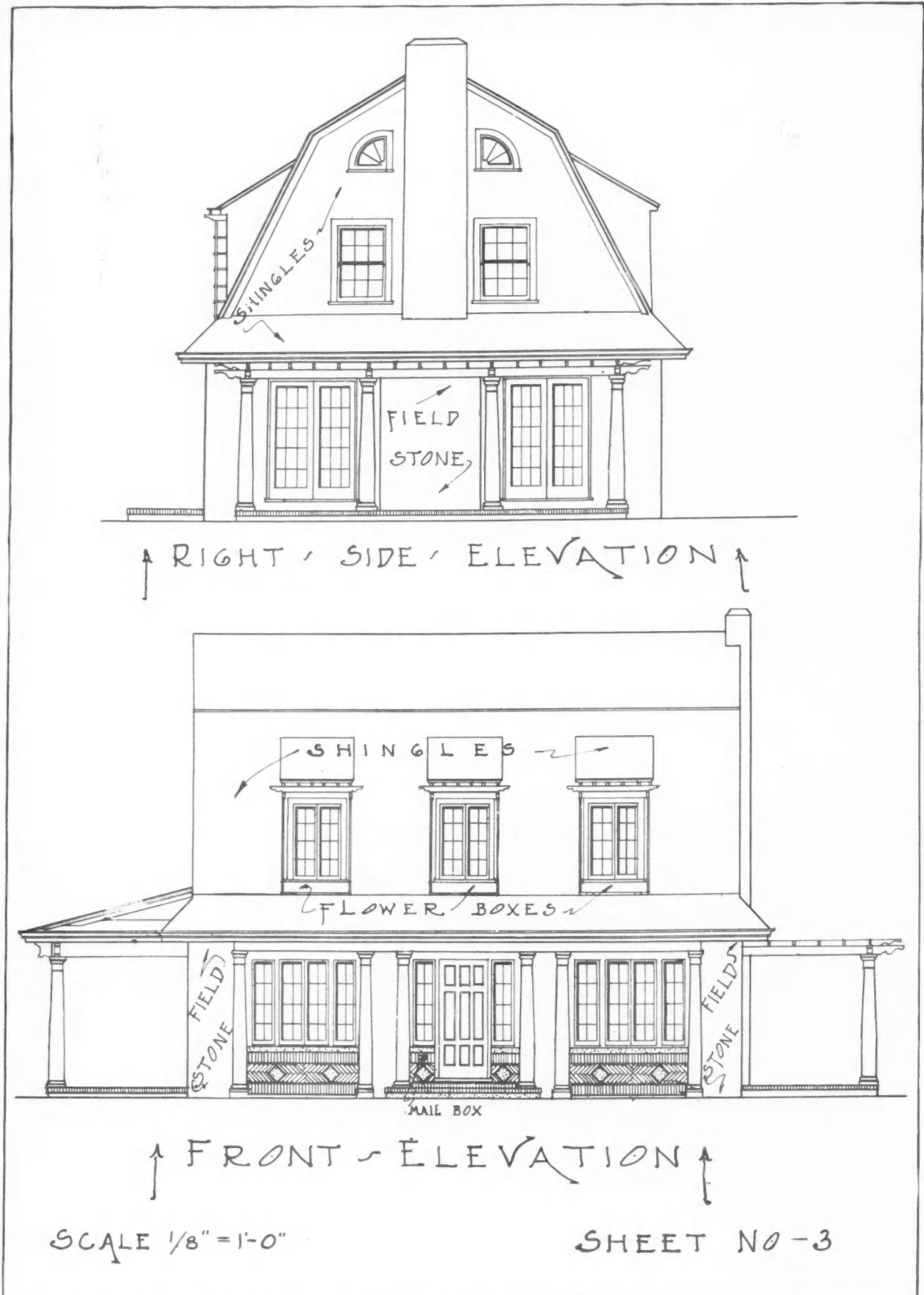
Front and Right Side Elevations of Our Front Cover Home Showing the Treatment of the Windows and of the Pillars Which Support the Porch Roofs and Are Carried Across the Front of the House.
