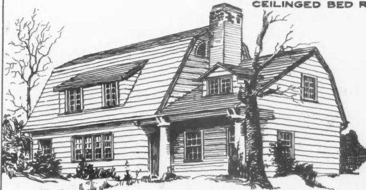
FIG. 6. ROOF & WALLS TO ACCOMMODATE A HIGH-CEILINGED BED ROOM.
