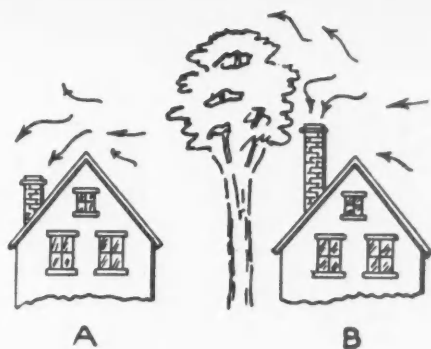
Fig. 1. Errors in chimney height That Are To Be Avoided. (A) Arrows indicate how wind drives smoke back down chimney when its top is below roof ridge. (B) When chimney tops are overshadowed by trees down draft occurs.
