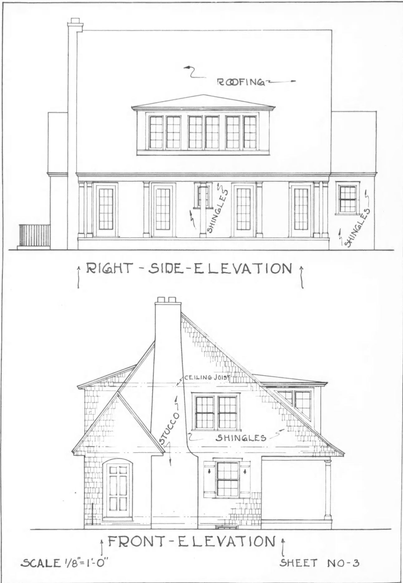
In the Right Side and Front Elevations of Our Front Cover Home, We See the Treatment of the Open Porch and the Sleeping Porch Above and Also of the Entrance and Chimney Details Which Face the Street.
