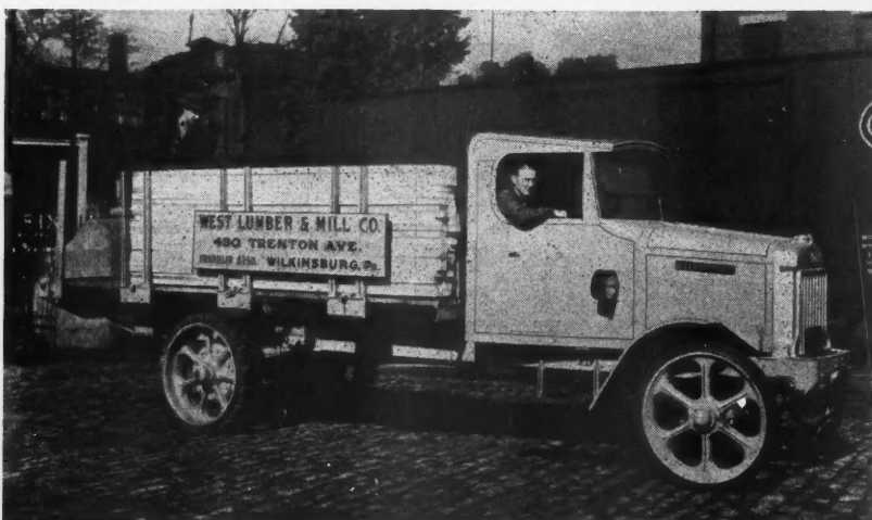
A Whole Truck Load of Lumber, Like This, Can Be Unloaded in a Few Moments When the Load Is Carried on Rollers Set Into the Platform, Making It Easy to Slide the Entire Load Off at Once.
