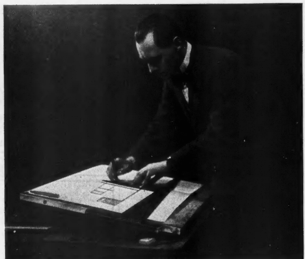
The Magnetic Head on This "Tee" Square Holds It Firmly Against the Drawing Board Leaving the Hands Entirely Free Thus Earning the Right to Be Described as a Third Hand.
