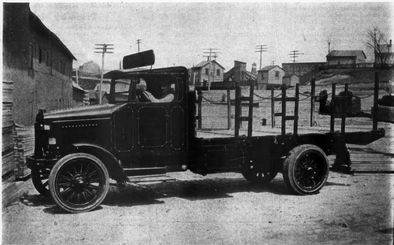
Here is a Lumber Truck with a Body Especially Equipped with Rollers for Quick Unloading. On the next page the same truck is seen loaded with lumber and another chassis, of the same model, equipped with platform body, is loaded with heavy bags of cement, a story of truck versatility in pictures.
