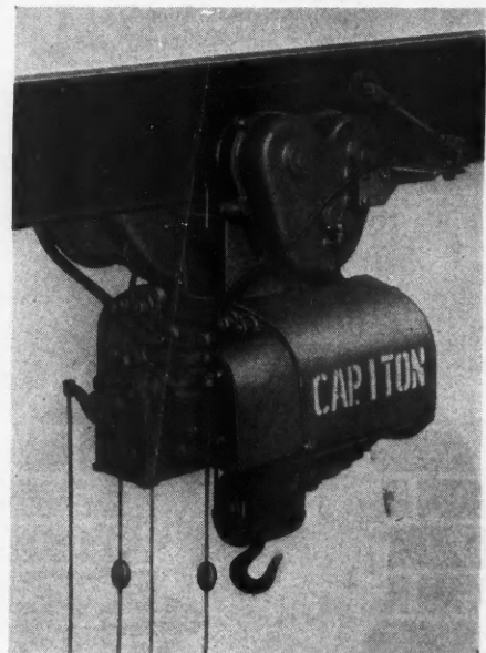
A Trolley Hoist Which Is Very Efficient in Spotting Work Because of Its Accurate Control.
