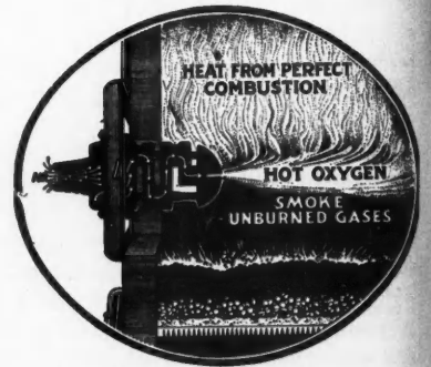
This Method of Supplying Heated Air to the Fire Bed Increases the Efficiency of the Furnace.
