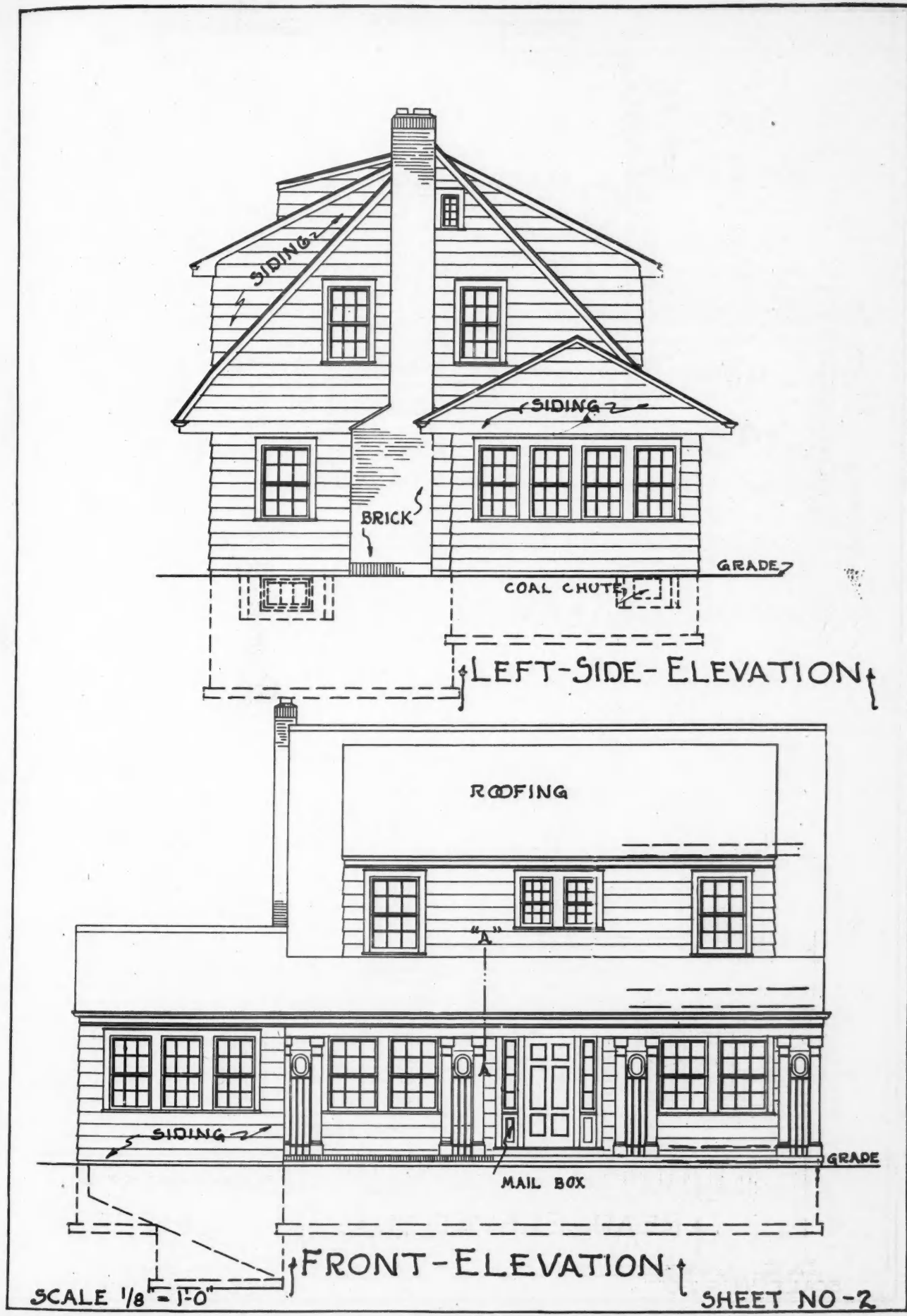
In Front and Left Side Elevations the Treatment of Roof Line, the Fireplace Chimney, the Pillared Porch and Sun Parlor Are Shown While on the Following Pages Further Details Will Be Found.
