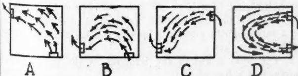
Fig. 3. The Arrows Show the Paths of Air Travel in Upward and Downward Air Distribution Systems.
