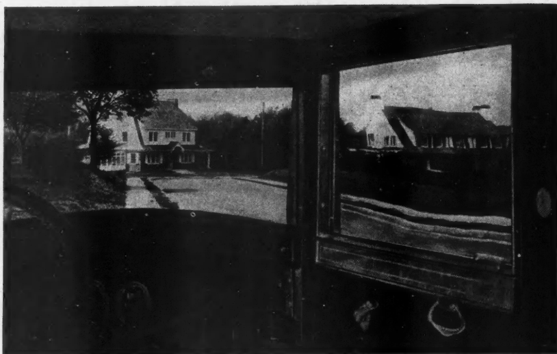
The Windshield Is Glazed with Plate Glass, the Side Window with Ordinary Glass. Here is a striking example of the better vision obtained when plate glass is used.
