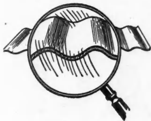
Two surfaces of Pure Lead seal a core of special analysis, copper content steel.
