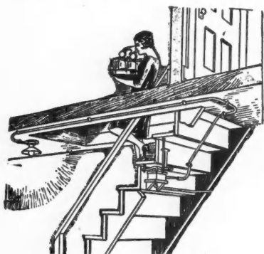
Automatic Control of Basement, Attic or Other Lights with a Switch in the Stair Tread.
