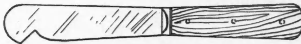
An Ordinary Putty Knife, Ground as Shown Here, Is a Handy Tool When Working with Roll Roofing or Asphalt Shingles.
