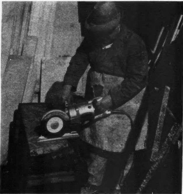
This New, Power, Hand Saw Is Designed for Cutting All Kinds of Stone and Similar Materials Rapidly and Economically.
