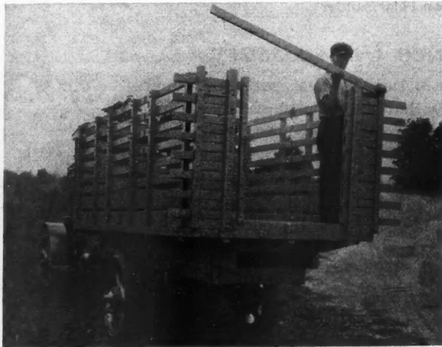
A Very Good Type of Body, Solid Floor with Movable Sides, a High Type for Stock Handling.
