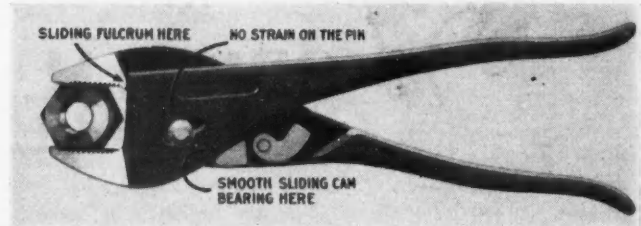
Something Really New, Pliers That Do the Work of Several Wrenches.
