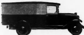
The new Chevrolet six-cylinder 1½ Ton Truck Chassis equipped with Panel Body
