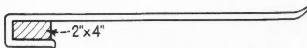
A Pipe with a Chisel Welded Into One End for Cutting Form Wires Below Ground and an Improved Wrecking Bar.
