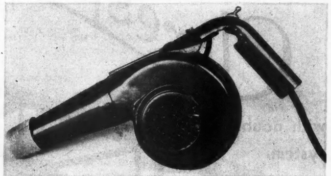
In Drilling Masonry and in Various Other Work, a Small Electric Blower Is a Time Saver to the Builder.
