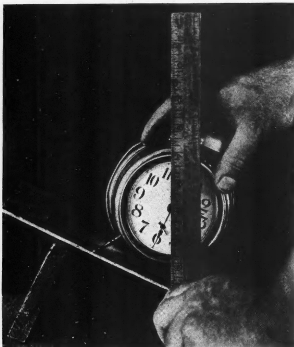
Using an Ordinary Alarm Clock to Lay Off a Thirty Degree Angle When Tools Are Not at Hand.
