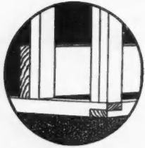
1. Plates and corner posts.
