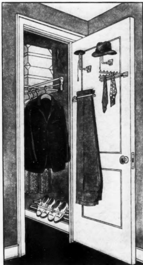
LEFT: Example of narrow and deep closet equipped with proper fixtures to give maximum capacity, convenience and proper storage of various items. The fixtures are described in text above.
