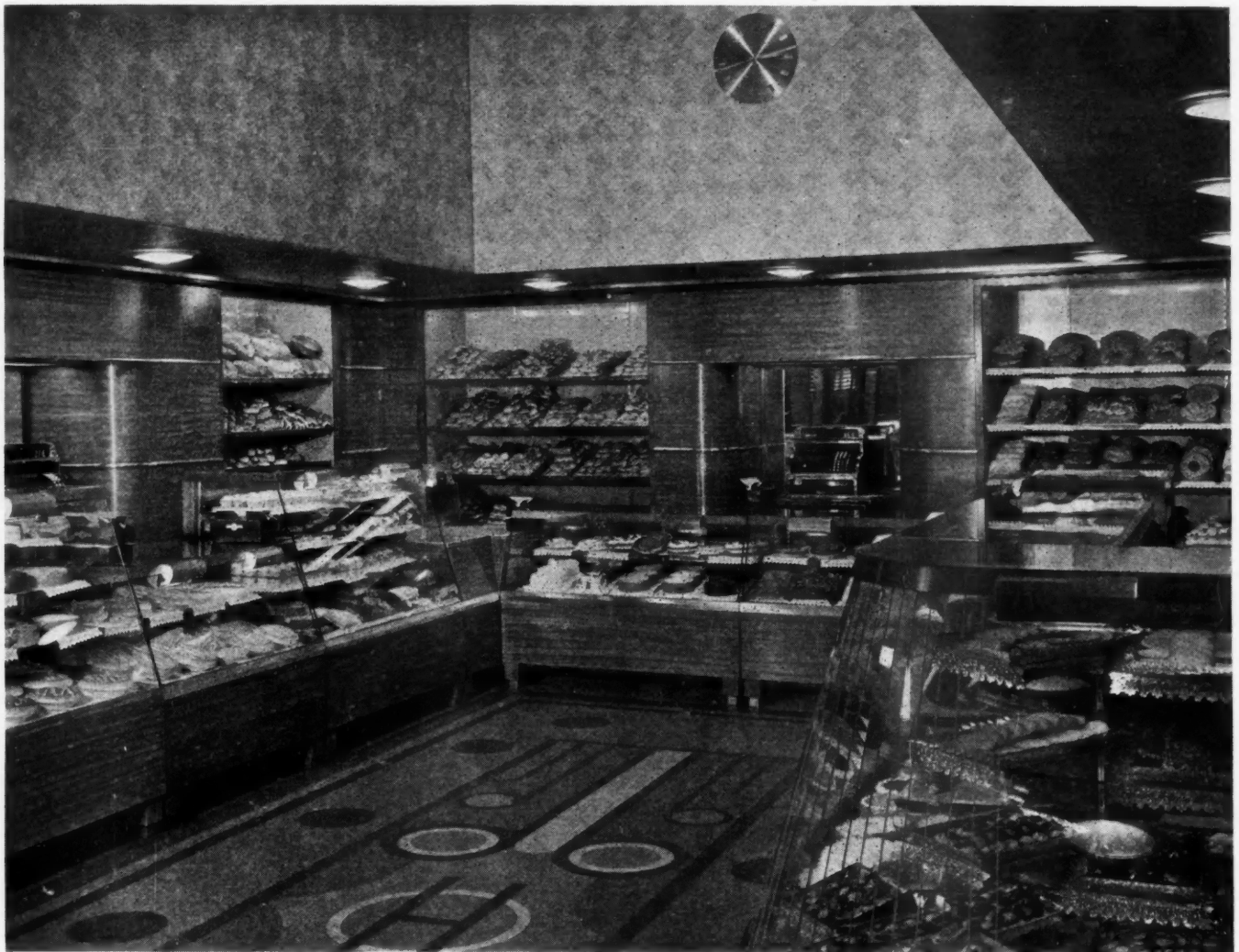
MODERN Hanscom bake shop interior features terrazzo floors, concealed lighting and walnut plywood paneling with snap-on mouldings.
