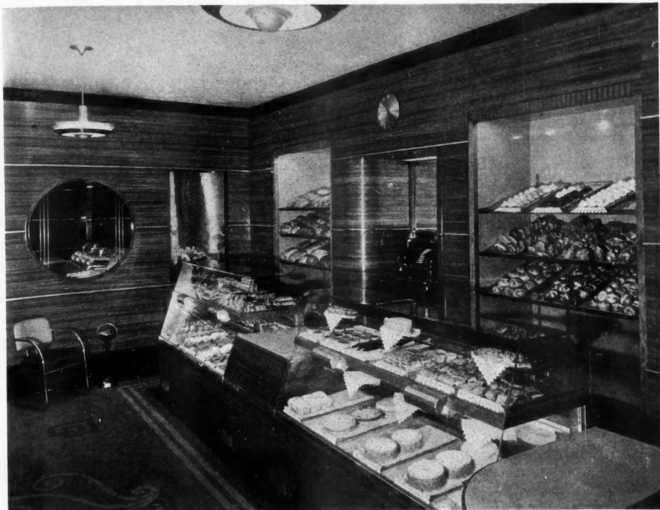
SMALL SHOP INTERIOR executed in modern design has display racks set in niches in wall; concealed lighting on bakery goods displayed.
