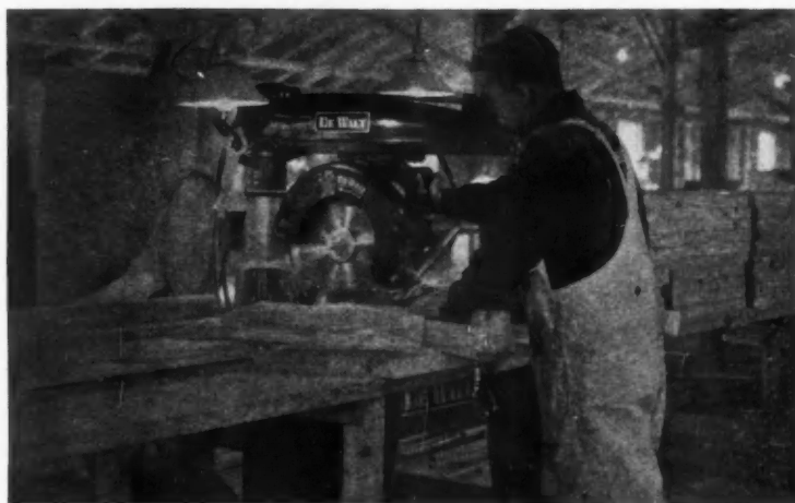
CUTTING CANOPY BRACES at Fort Devens. A saving of $163 was made in this one operation; other savings are listed in article.
