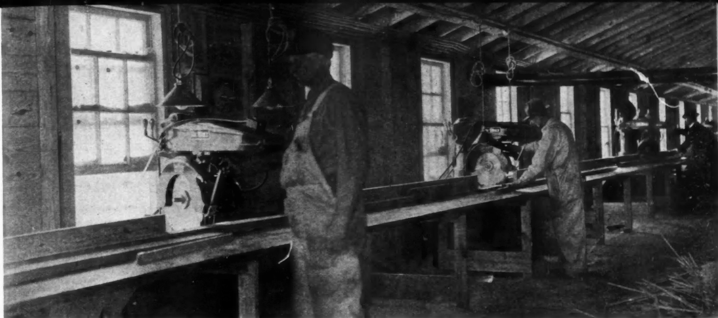
THIS FOUR-SAW straight line rafter cutting setup is used by Coleman Brothers and John Bowen, Inc., at Fort Devens, Mass. Lumber is squared off on first saw, moved on to second for the angle cut, then to the third for the first heel cut, then to the fourth for second heel cut.
