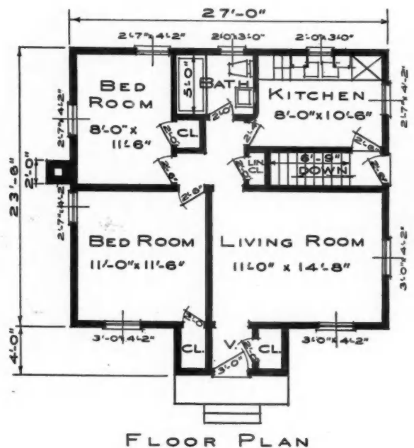
FLOOR PLAN of Type 1 Speedway Home, illustrated above, is 27' x 23' 6", with a 14' 8" x 11' living room. House has full 7' basement. Economical kitchen and bathroom plumbing layout is indicated at left.
